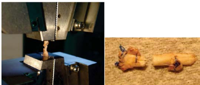
Figure 4. Typical mode of failure into the mid-substance of the autograft tendon
